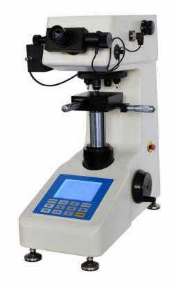
iVick-457HK Digital Micro Vickers hardness tester is a high-tech and new product combining the optics, mechanic and electrics features.
